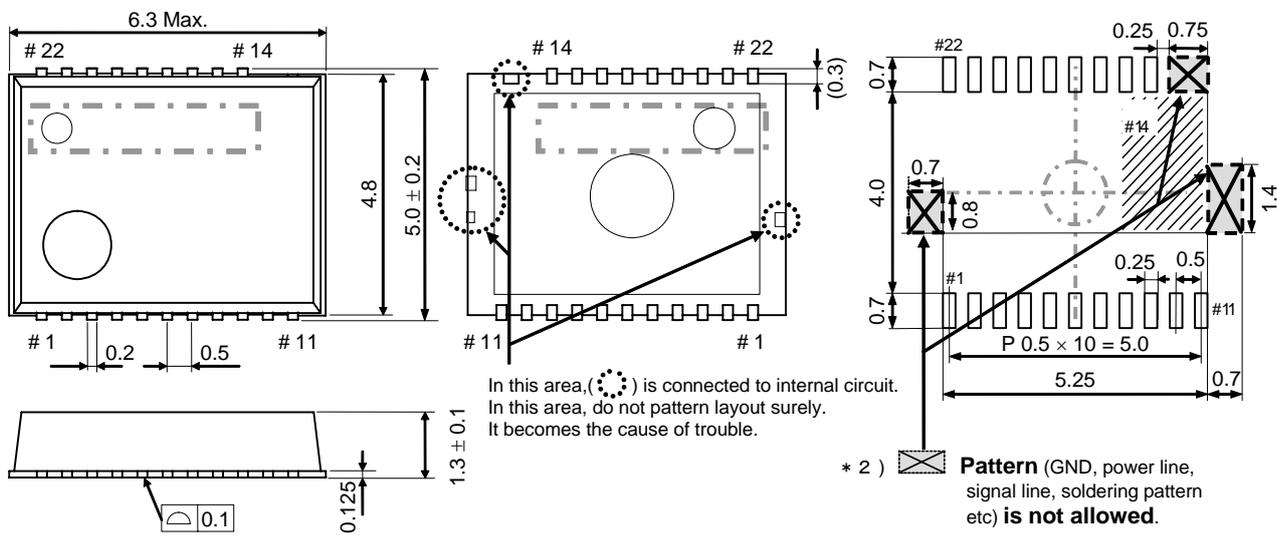
In this area, (
