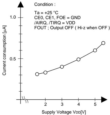
(3-2) Current consumption when non-accessed (ii) when FOUT=32.768 kHz
