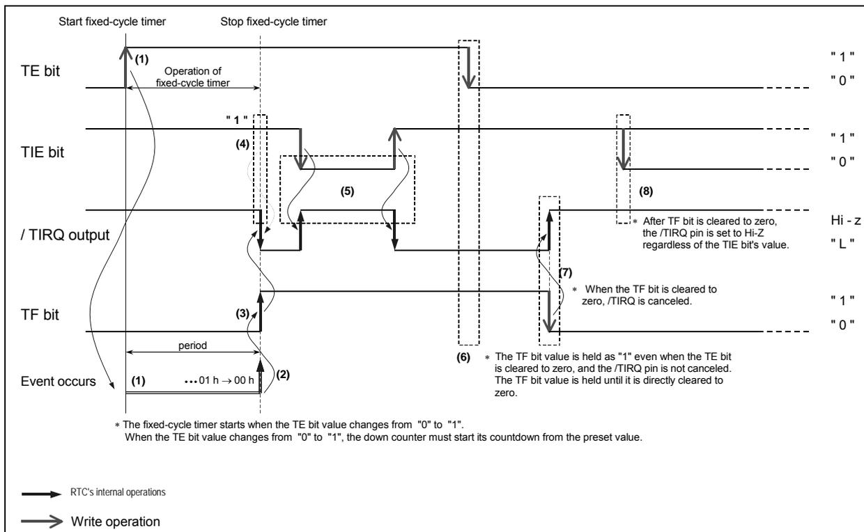
\*) Before using level interrupt mode (TI / TP = "0") , be sure to clear the TE bit and the TF bit to zero each time.
