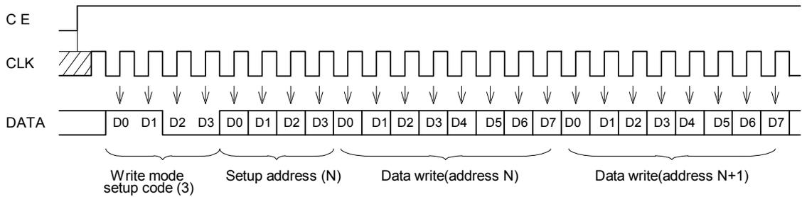
\* When writing data, the data needs to be entered in 8-bits units. If the input of data in 8-bits unit is not completed before CE input falls, the 8-bits data will not be written properly at the time CE input falls.
