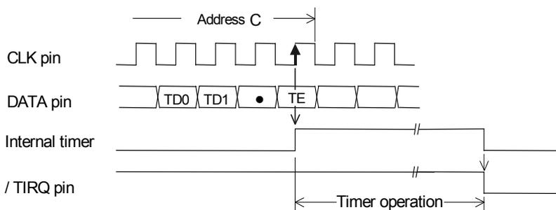
13.2.3. Fixed-cycle timer interrupt interval (example)
