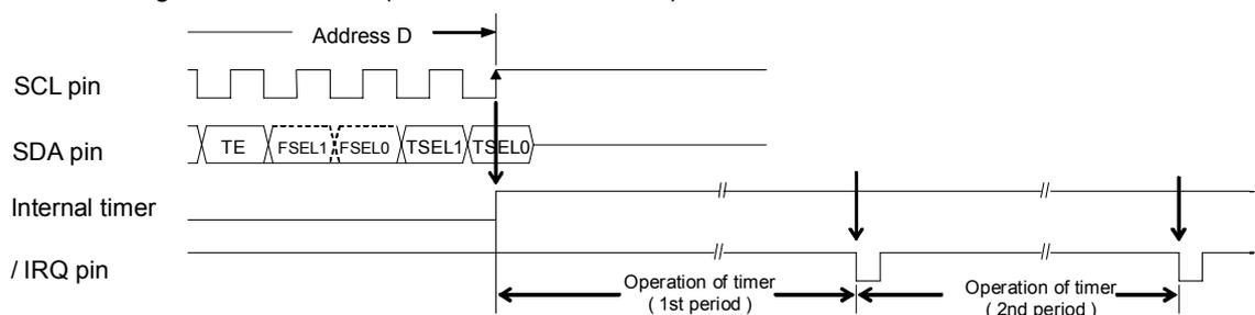
13.2.4. Fixed-cycle timer interrupt interval (example)
