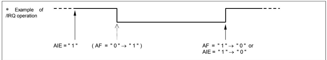
13.3.1. Diagram of alarm interrupt function
