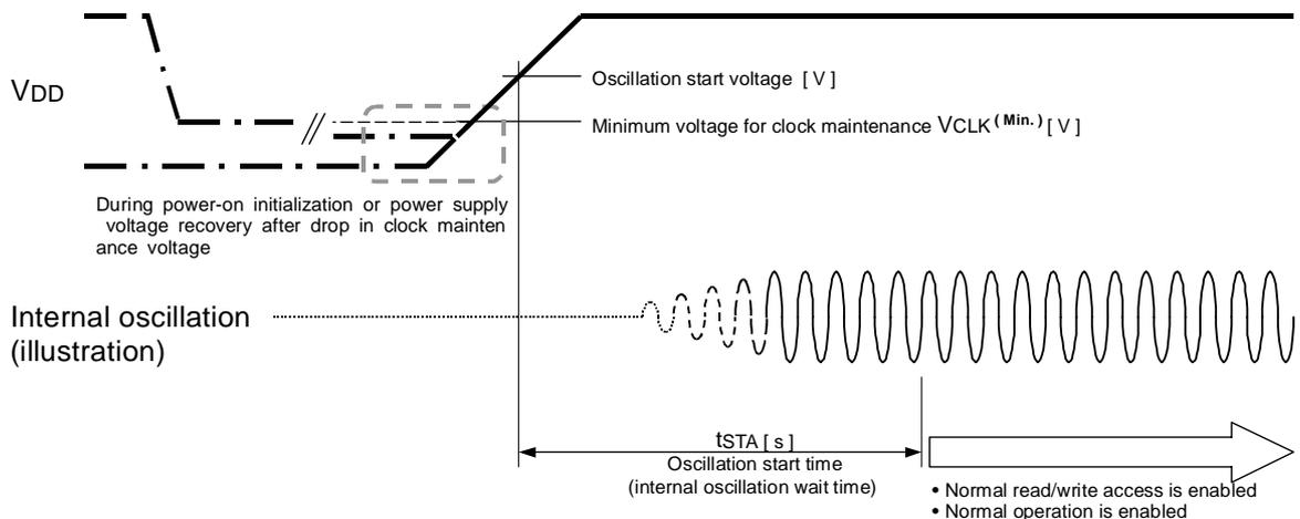
3) When the read VL-bit value is "VL = 0 (normal status)", access is enabled without waiting for stabilization of oscillation.
