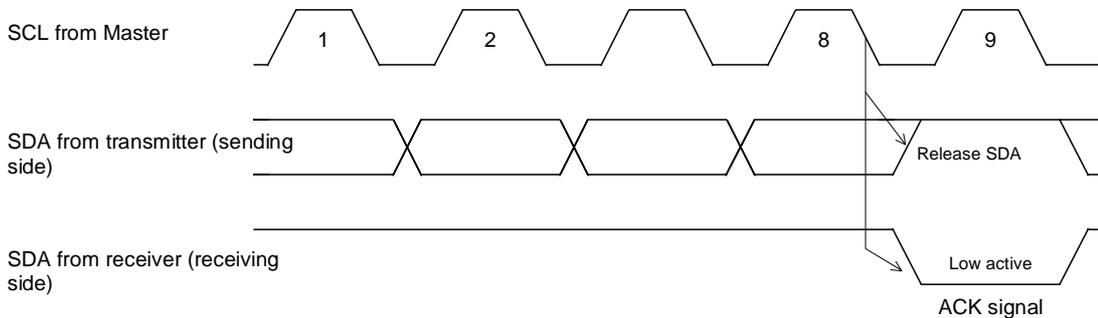
After transmitting the ACK signal, if the Master remains the receiver for transfer of the next byte, the SDA is released at the falling edge of the clock corresponding to the 13th bit of data on the SCL line. Data transfer resumes when the Master becomes the transmitter.
