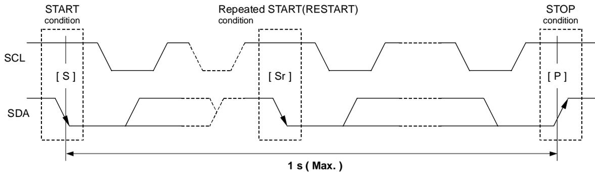
1) START condition, repeated START condition, and STOP condition
