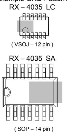
\* The shaded part ( ) indicates where a GND pattern should be set without getting too close to a signal line
