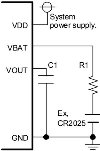
Case of secondary battery connection. And charge voltage = system supply voltage.
