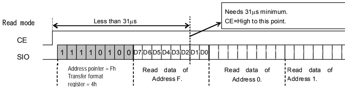
Incorrect example 3: If interval between two time read operations is less than 61 μs
