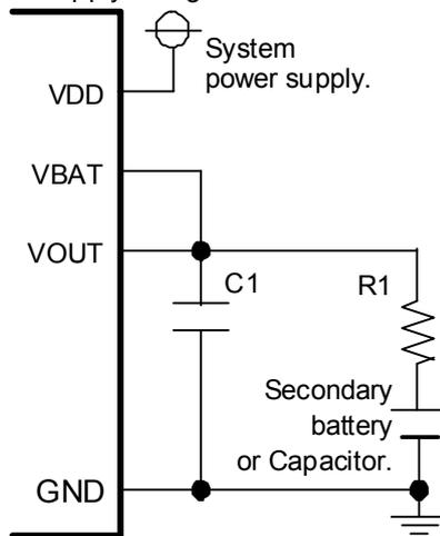
Case of secondary battery connection when the main power supply voltage is different from the charge voltage.
