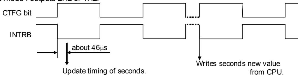
In a pulse mode, update of seconds is behind with about 46µs from a falling edge of INT.
