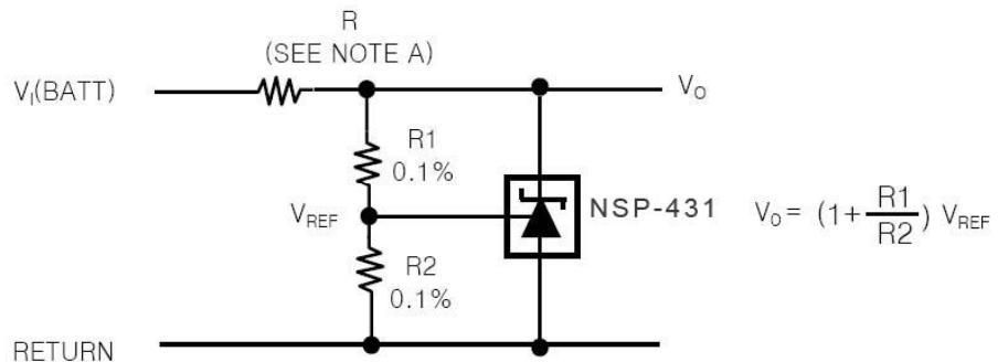
Note A : R Should provide cathode Current 1mA to the NSP-431K at minimum  $V_I(BATT)$
