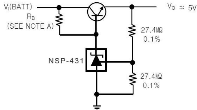
NOTE A : RB Should provide cathode Current  $\geq 1mA$  to the NSP-431K.
